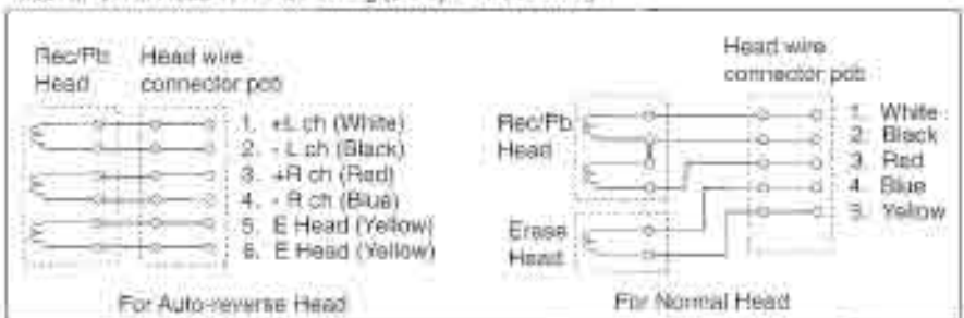
Mechanism B Head Wires Soldering (Dolby B NR version)
